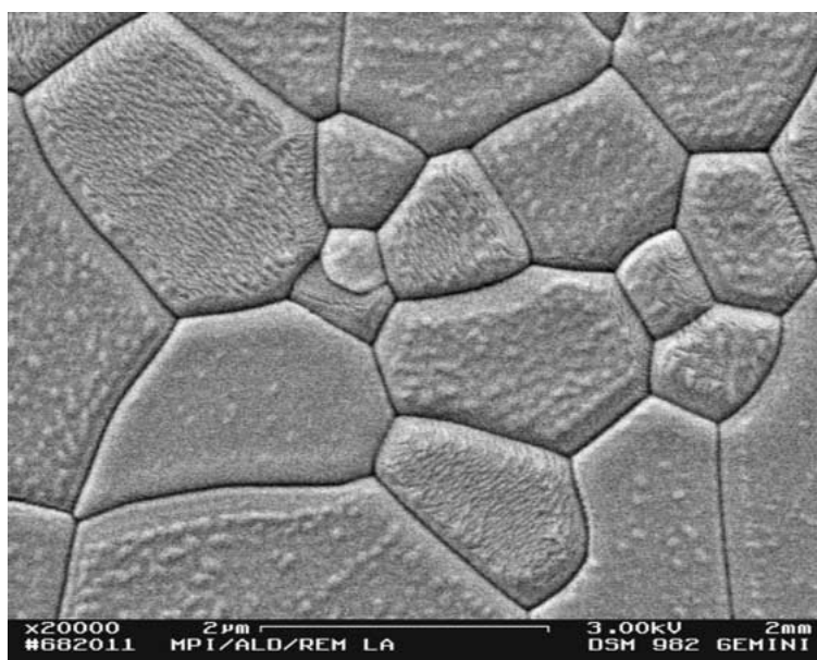
Figure 2 Microstructure of sintered (8 mol% \text{Y}_2\text{O}_3 ) \text{ZrO}_2 .
